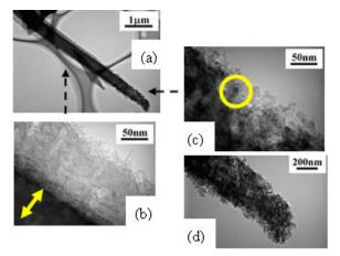
Studies by Okuno and colleagues suggest that nanocrystals are responsible for the red photoluminescence in silicon nanowires. Transmission electron microscopy images show a silicon nanowire (a), a zoom in on the interface between silicon crystalline core (arrow) and surrounding silicon oxide in the middle part of the nanowire in (b) and a zoom in on the top end (c) and (d). The circle in (c) shows an example of silicon nanocrystals.
